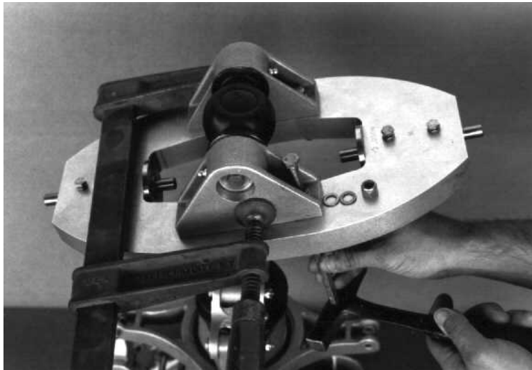
Photo #4: Drive out the teeter block bolts.
